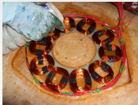
The PM rotor, the stator cast in resin, assembly and the finished generator - photos ESCANDA Spain
