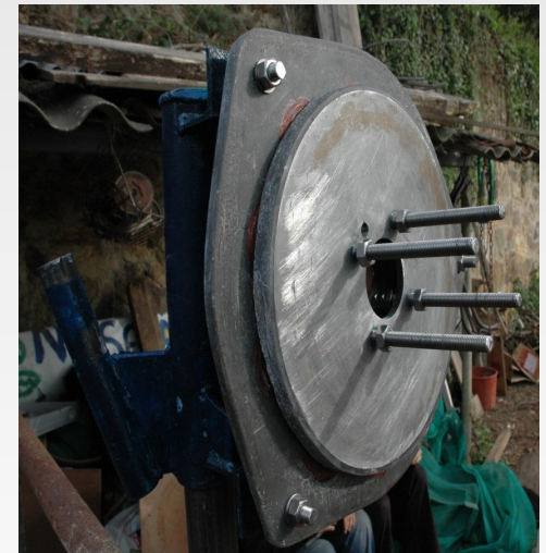
The PM rotor, the stator cast in resin, assembly and the finished generator - photos ESCANDA Spain
